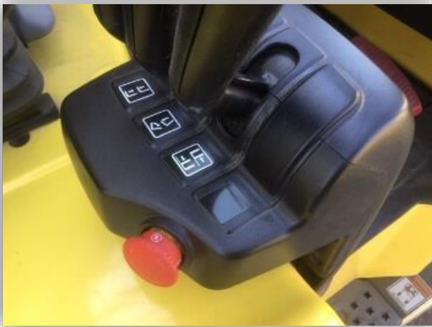
Hyster E60XN "E" Stop Button rotate and pull outward to power on truck.
