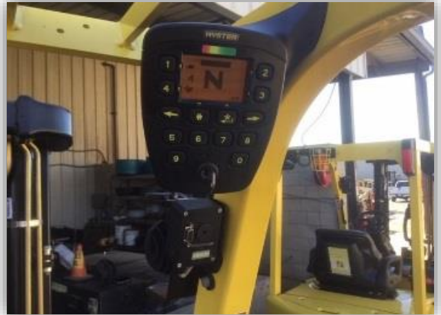
Hyster E60XN mounted display with "KEY ON" position truck in neutral park condition.
