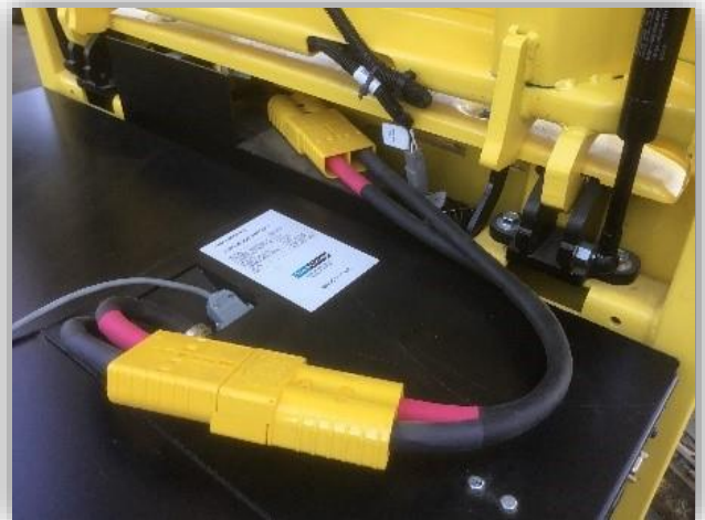
Yellow SB Jumper Connectors Shown Connected Correctly. Do Not Disturb!
